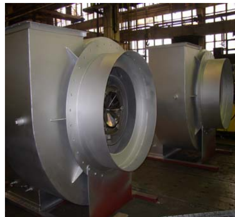
Hamworthy Low-calorific gas burner for firing Waste gases
