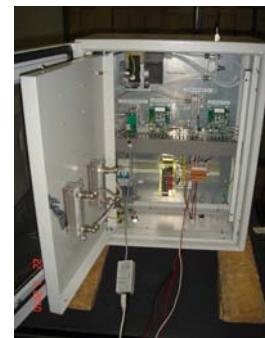
Analyser Unit Internal View
